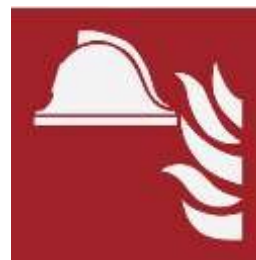
Means and equipment for fire fighting
